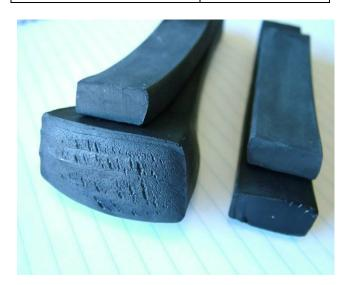
**Left** – Expansion in fresh water compared to original product. **Right** – Expansion in salt water compared to original product.
