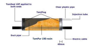
TamPur 190 is based on a polyol component (Part A) and a prepolymer of polyurethane (Part B). The polyol component has been degassed to help reduce foaming during the reaction with the polyurethane prepolymer, giving a hydrophobic injection resin.
